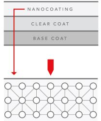
When the coating is lightly scratched, the elastomers compress instead of breaking.
